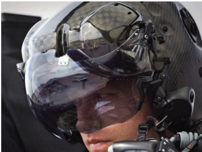
The DAS collects imagery from six infrared (IR) cameras mounted around the aircraft and sends it to the pilot's helmet-mounted display for a 360-degree spherical view of the environment.
